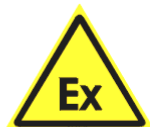
Fig. 2 Danger - Explosive Atmosphere
