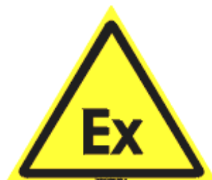
Fig. 2 Danger - Explosive Atmosphere
