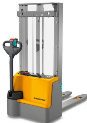
Fig. 2. Example of an electric pedestrian-controlled lift truck
