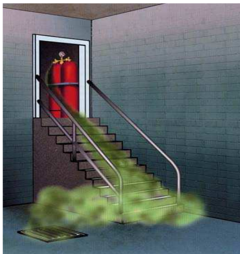
Fig. 7. Possible places of accumulation of gases which are heavier than air
